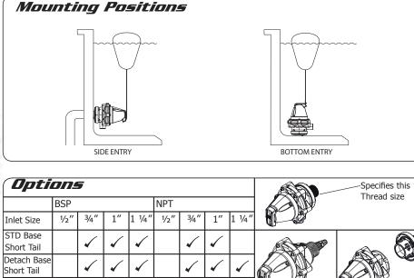
Long Tail Available only with Detach Base. Supplied with backnut and seal washer. 1/2" Long Tail: 100mm long. 3/4" Long Tail: 38mm long.
