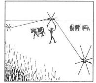
Lift Tumblewheels up *vertically* to allow stock and machinery to pass underneath wire.
