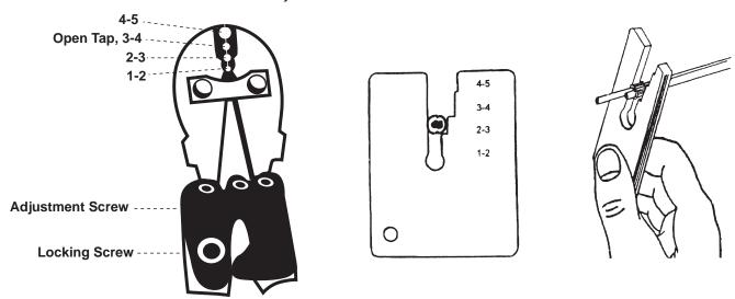
With handles open, loosen locking screw with Allen wrench one or two turns. Turn adjustment screw clockwise about 1/4 turn. Tighten lock screw then make a press check with gauge. Repeat as needed until gauge easily passes over pressed sleeve.
