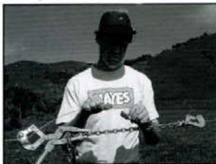
FOR A CENTRE STRAIN (gut strain) attach each grip towards the ends of the wires leaving sufficient wire to join either over, or in front of the strainer.
