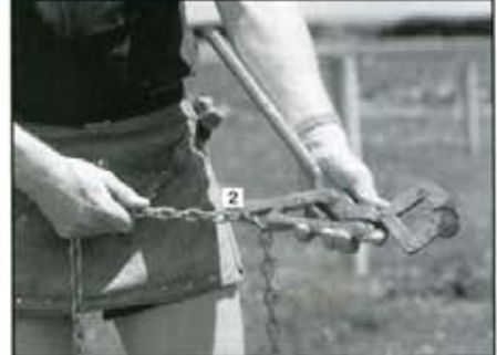
2: Insert the chain into the strainer grab [2]. Run the chain of the H300 through your hand to remove all twists from the chain.
