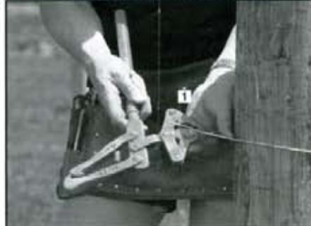
USING A WIRE STROP 1: Attach grip [1] of strainer to strop by opening grip and inserting strop.
