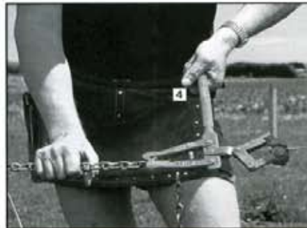
4: Continue to remove any slack by operating the handle [4] in a levering action until the desired tension* is reached. Tie off wire.
