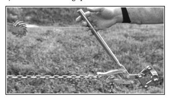
Remove slack in fence wire by operating handle in a ratcheting action.
