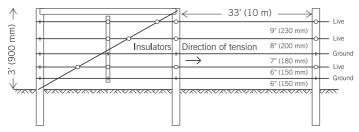
H-Brace — Very simple to erect and most suitable as a high tension strainer, excellent in areas where the soil gets very wet or where heavy frost occurs.
