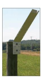
Attach bracket to wood post with two 3/8" x 4" lag screws (included). **Note:** Additional holes on base of bracket allow mounting on pipe, t-post, etc. using either hose clamps or 2 1/8" U-bolts (not included).
