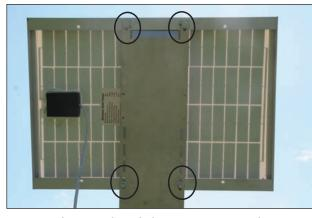
Center the panel and then secure it to the bracket with four self-tapping screws (included) as circled. Use the slots on the bracket to determine screw placement.
