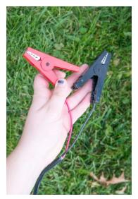
\*Remove the alligator clips from the energizer, and mark the positive and negative wires prior to removal. Strip the insulation from the wire ends. Splice the alligator clip ends to the corresponding charge controller load wires.
