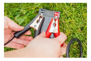
**<u>Step 3</u>**: Connect Panel A's negative (bottom) plug to the charge controller's negative (black) plug.
